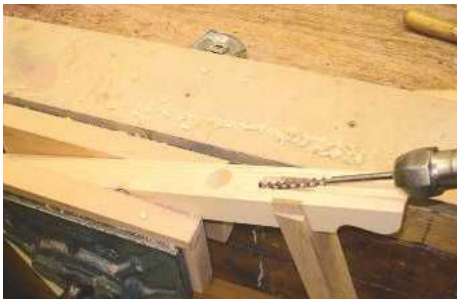
▲ Pic.25 Two holes need to be drilled, one 8mm hole for the cord and one 32mm hole for the knot
